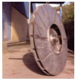
designed and constructed a special test rig so that the testing could be completed in-house. Part overlaying the mild steel shaft with Hastelloy® ensured corrosion resistance in the contact area and cryogenic cooling of the shaft and impeller was required to shrink the shaft sufficiently to fit into the fan centre boss. The result, upon returning to ambient temperature, was a unified shaft/impeller assembly that was then precision balanced in-house and shipped as one complete unit.
